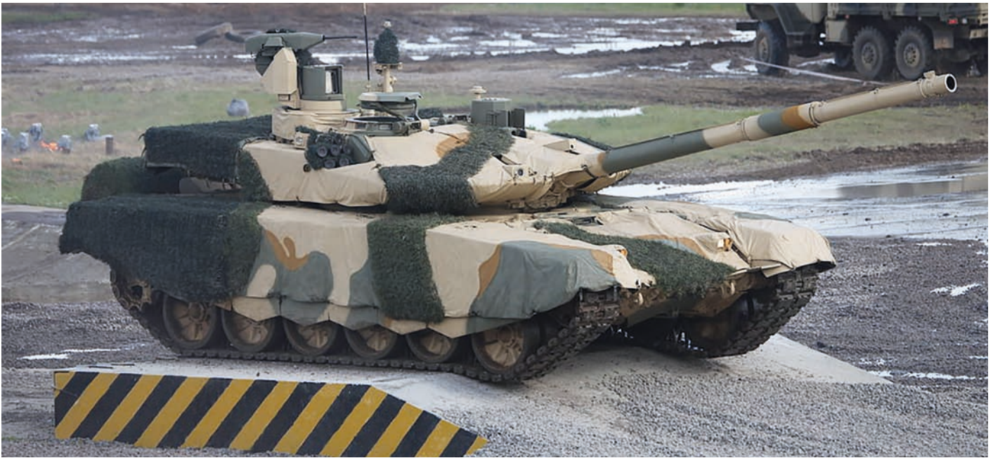
Some MBT, like the Russian T90MS, feature an RWS to replace the open mount commander's hatch weapon. The T90MS RWS appears to be aimed by the commander's panoramic sight. (Photo: AI)
